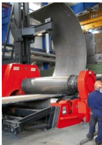
Figura 2-7 - Chapas de aço a tomarem forma cónica (Wind Power Engineering & Development, 2015).
