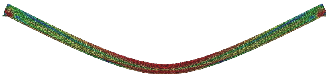
Figure 6.19 - Simply supported purlin at the moment of failure
