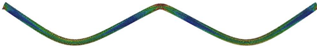
Figure 6.20 - Continuous two-span purlin at the moment of failure
