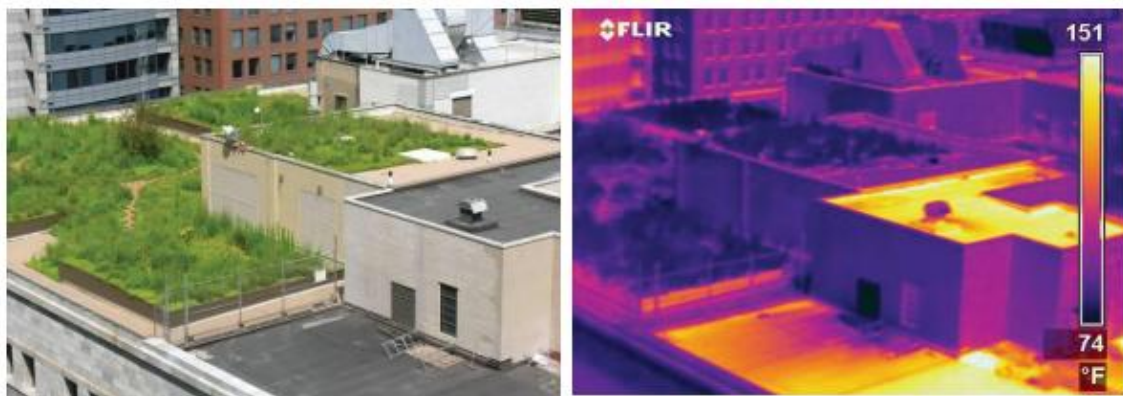
Figure 2.11 - Thermal scan of a conventional roof and a green roof (EPA a, 2008).
