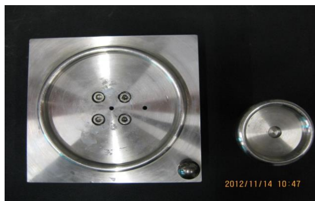
Figure 4.6 – CDR rings ( r = 40 , r_2 = 80 ) and sphere [5.]
