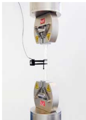
Figure 1.5 – Test setup with the Acrylate specimen and dynamic extensometer [29.]
