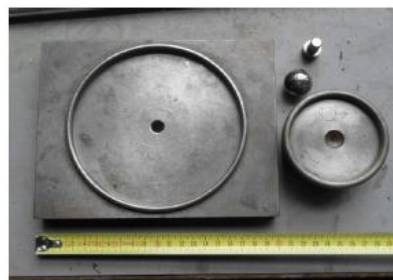
Figure 1.6 – CDR bending test: load ring, r=43\text{mm} ; support ring, r=72,5\text{mm} [13.]
