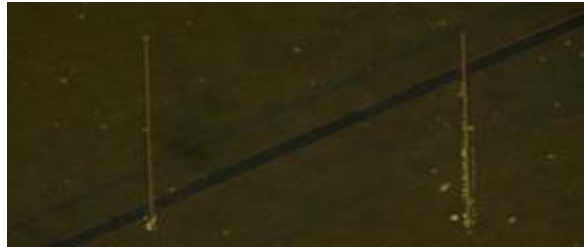
Figure 4.8 – 1 Induced flaws (100 x magnified)
