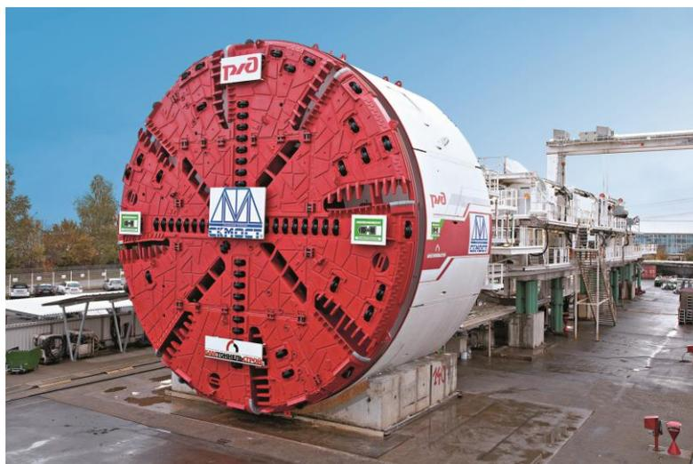
Figura 3.11 – *Single Shield* TBM (Herrenknecht AG@, 2014).
