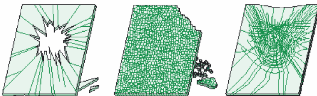
Figure 2-Fracture behavior of annealed, toughened and laminated glass respectively[5].
