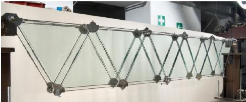
Figure 3.6 – Hybrid pre-stressed steel-glass beam (Froli & Lani, 2010)
