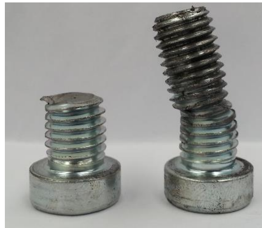
b) Socketed head bolt sheared
