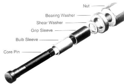
c.1) Exploded view of Huck Ultra-Twist bolt
