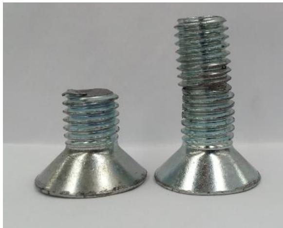
a) Countersunk bolt sheared
