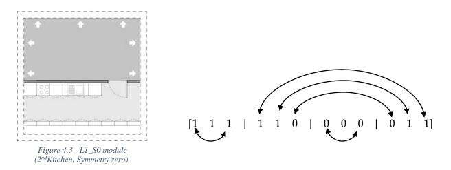
In this case: (i) the order of the first terms inside the sub-matrix is inverted, and similarly for the third one; (ii) the order of the other two sub-matrices is also inverted, but these two sub-matrices also swap their position.
