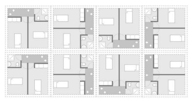
Figure 3.4 – Example of the 8 possible transformations of a module (R1\_R0).
