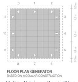
*Figure 3.2 - General*  $6x6m^2$  *area, with a grid of* 0,6m *per unit.*
