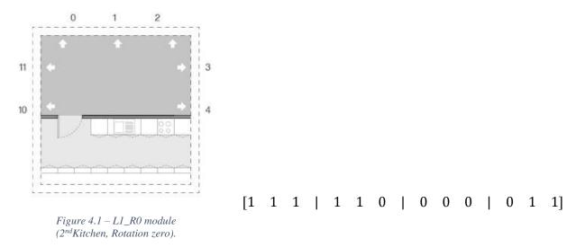
It can be seen that: (i) the matrix is subdivided into four ordered sub-matrices, corresponding to the north, east, south and west sides; (ii) for each side of the module three possibilities for door locations exist, showing a "1" if there is an opening and a "0" otherwise.
