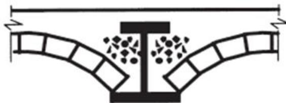
Figura 4 - Sistema *Jack-arch* [9]
