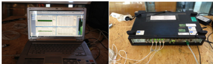
Figura 3.9 - Sistema Multi-analisador Pulse TM, com o Software PULSE LabShop Version 15.1.0.
