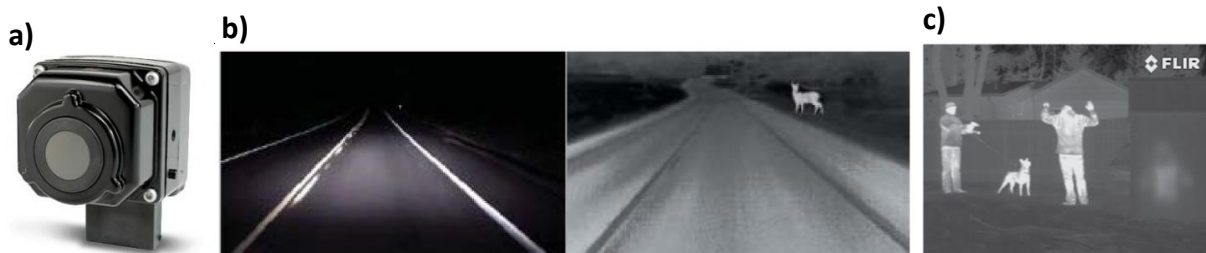
Figure 4.4 - a) FLIR Camera; b) comparison between road visibility with regular headlights; c) example of law enforcement use (FLIR, 2008).
