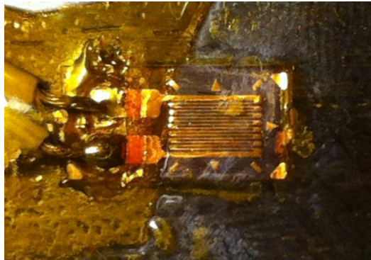
Figure 3.5. Strain gages glued to the composite plate.
