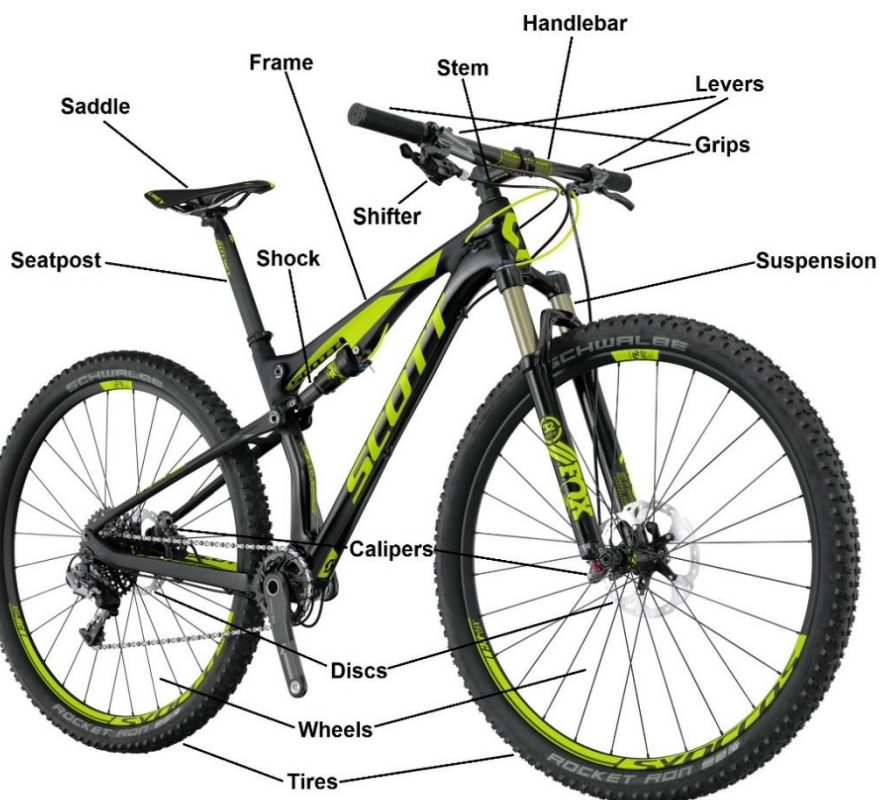
Figure 2.11. Scheme of the components on a Scott mountain bicycle.
