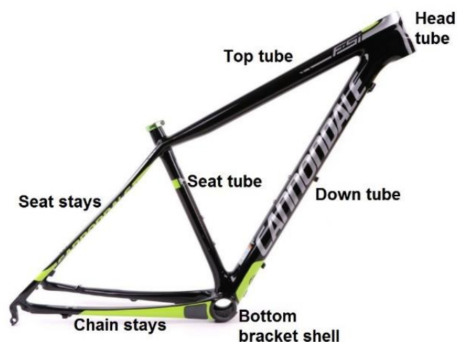
Figure 2.12. Scheme of the tubes on a Cannondale mountain bicycle frame.
