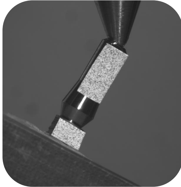
Fig. VI A sample being tested in the test-machine (AG-I Shimadzu) using a pointed tip.
