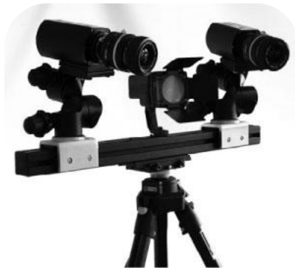
Fig. V DIC 3D camera setup.
