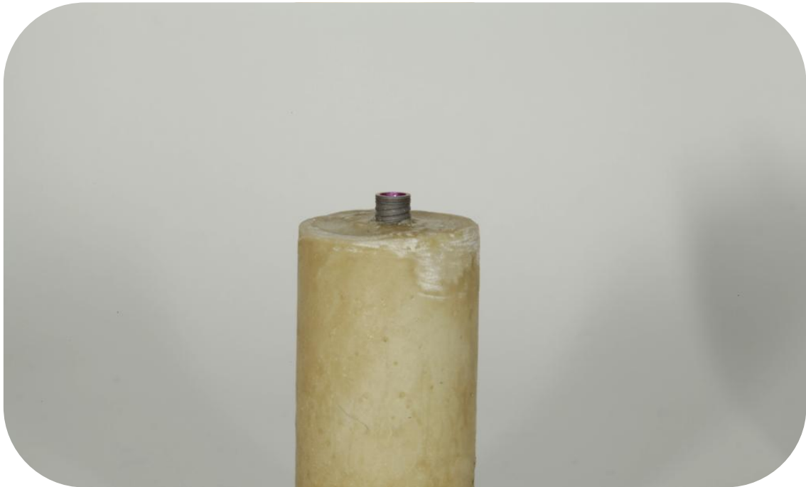
Fig. III The molds obtained from the inclusion of the implants in the resin.
