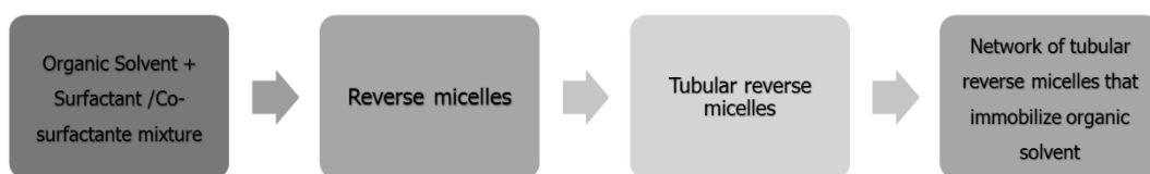
Figure 17 – Formation of organogels by fluid-filled fiber mechanism.
