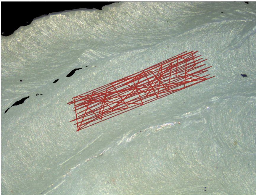
Image 4 – Example of an aleatory path made to calculate the surface roughness parameters; it's located between the relief marks, to eliminate the shape factor, which can produce misleading results.
