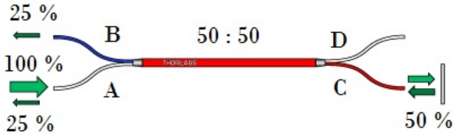
Figure 29: Schematic of a 50:50 split ratio fiber optic coupler, used as circulator. Adapted from [26].
