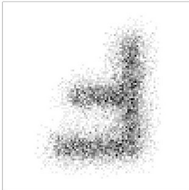
Figure 63: Image simulation for the scanning objective lens LSM04–BB , showing the consequences of spherical aberration. Results from Zemax OpticStudio 15.
