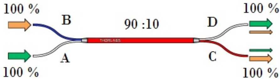
Figure 28: Schematic of a 90:10 split ratio fiber optic coupler, used as interferometer. Adapted from [26].
