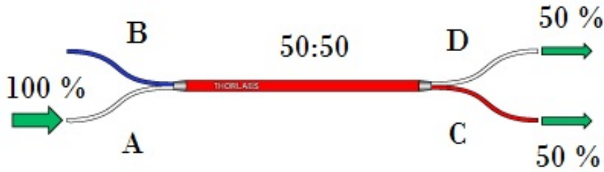
Figure 27: Schematic of a 50:50 split ratio fiber optic coupler, used as beam splitter. Adapted from [26].
