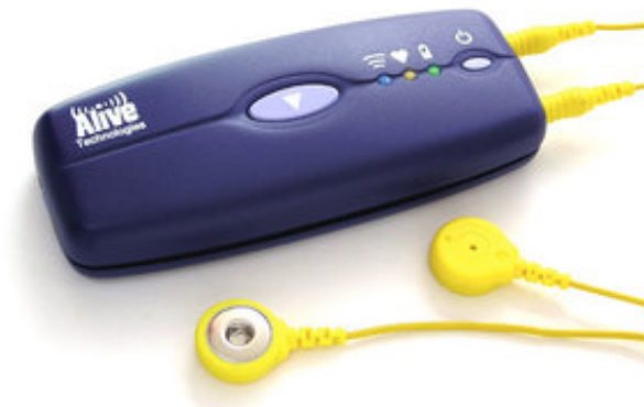
FIGURA 2.15: Hardware do Alive Bluetooth Heart & Activity Monitor[23].
