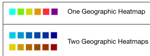
Figure 30 - Discrete color spaces used to color the Geographic Heatmaps when rendered to the Screen Buffer. The top is used when only one heatmap is rendered and the bottom is used when two heatmaps are rendered at the same time.
