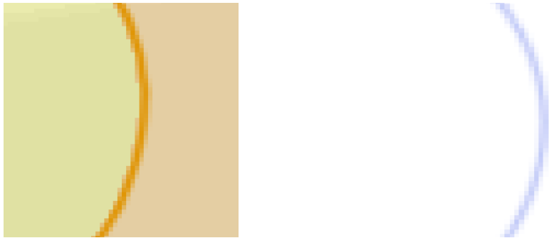
Figure 42 - Comparison between vertical curves. On the left a smooth line rendered by our application, and on the right a smooth line rasterized with Adobe Photoshop.
