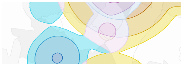
Figure 36 - Variation of color and the color's alpha value near the interpolated edge in order to render the anti-aliased line. Notice the purple color in the center, result of the blending configuration.
