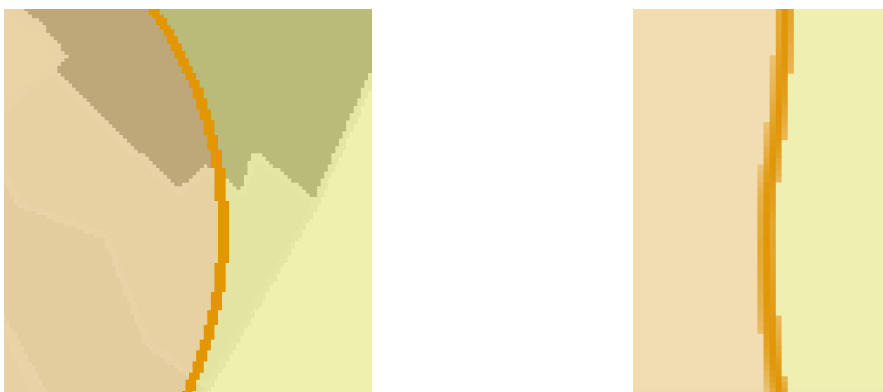
Figure 41 - Aliased line on the left, magnified. On the right an antialiased line obtained with our implemented algorithm, also magnified.
