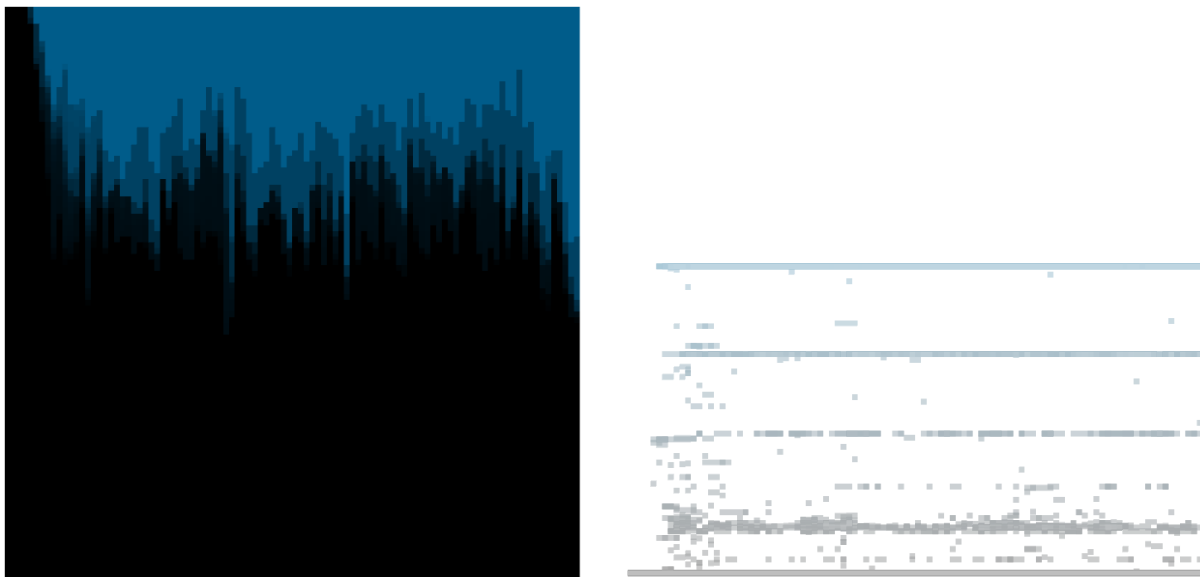
Fig. 5.29 Fitness view of an individual which was not able to create individuals with better fitness than each previous population after the first few generations. Because of elitism the current best kept being copied from each previous population, which can easily be seen in the position by fitness mode on the right, represented by the top horizontal line.
