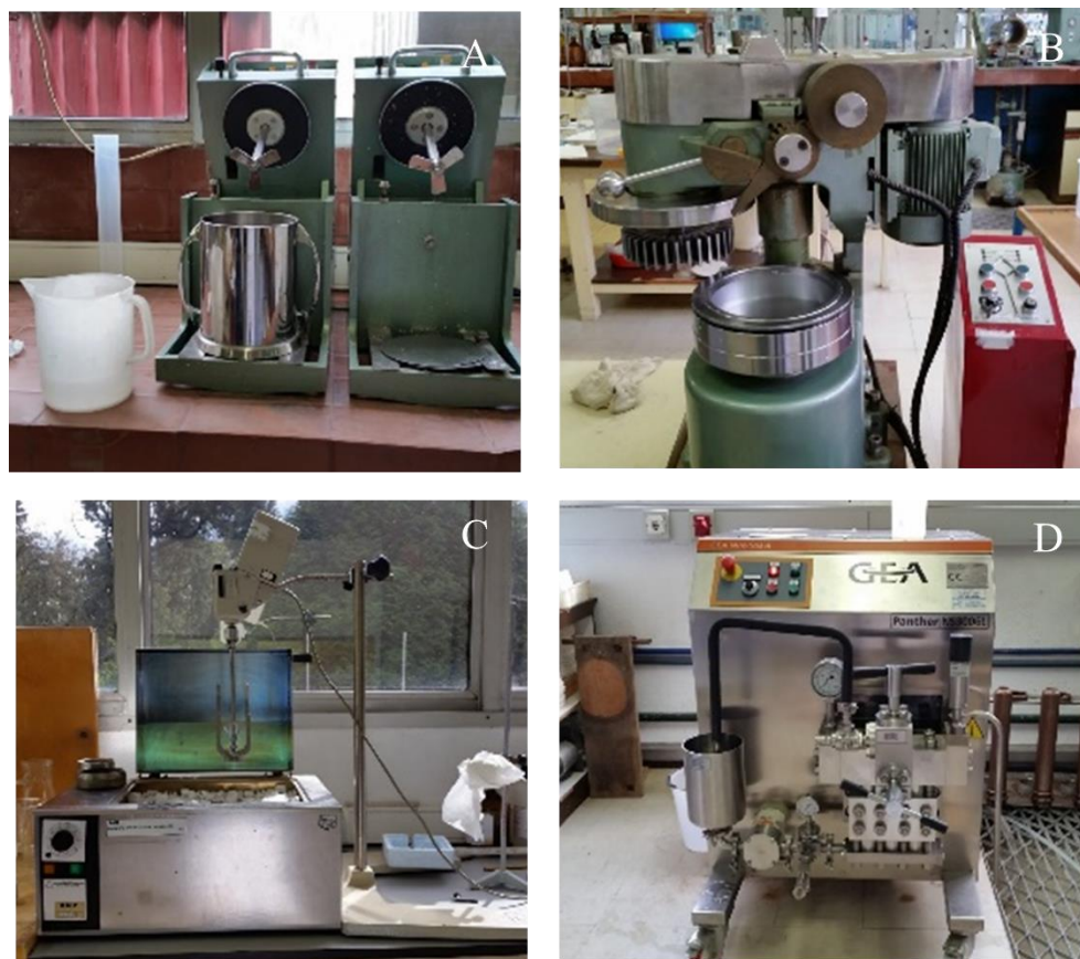
Figure 10. CMF procedure concerning the several steps of the process: (A) exposure of fibers to pulp disintegrator (B) pulp beating (C) enzymatic treatment (D) homogenization.
