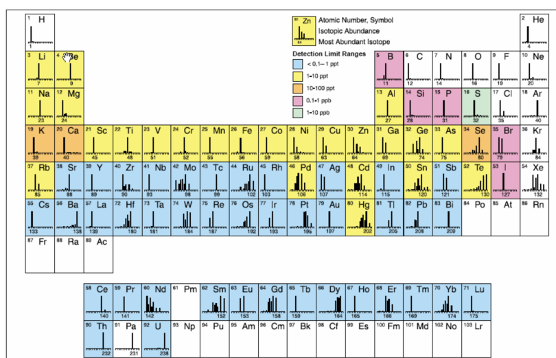
Figure 2.1: Approximate detection capabilities of the quadrupole ICP-MS. Adapted from [Bazilio and Weinrich, 2012].
