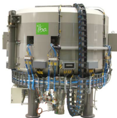
Figure 5.3: Cyclone 18/9 MeV from IBA.
