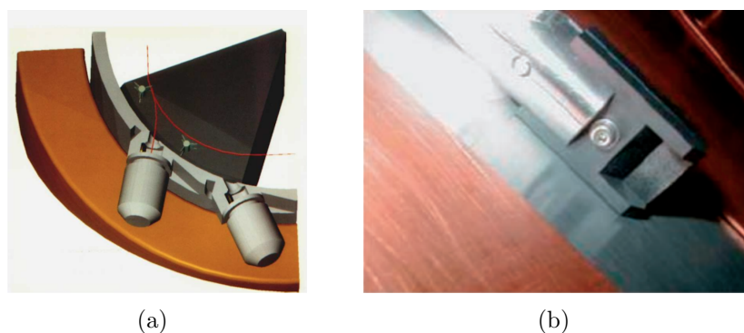
Figure 3.4: a) Schematic of multiple extraction ports in a cyclotron. b) Image of a thin carbon stripper foil.
