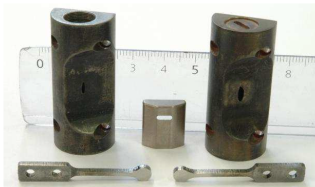
Figure 3.3: Example of chimneys, cathodes and puller. Two copper - tungsten chimneys at the back (note that the chimney on the right shows an eroded slit). Two tantalum cathodes up front (they are shaped to reduce heat conduction and the material allows for high electron emission). In the middle is a puller or extraction electrode, it is used to extract the beam from the ion source to the accelerating region inside the cyclotron. Its alignment with the chimney aperture is critical to the initial launch angle. Image adapted from [Kleven and Zarembo, 2015].
