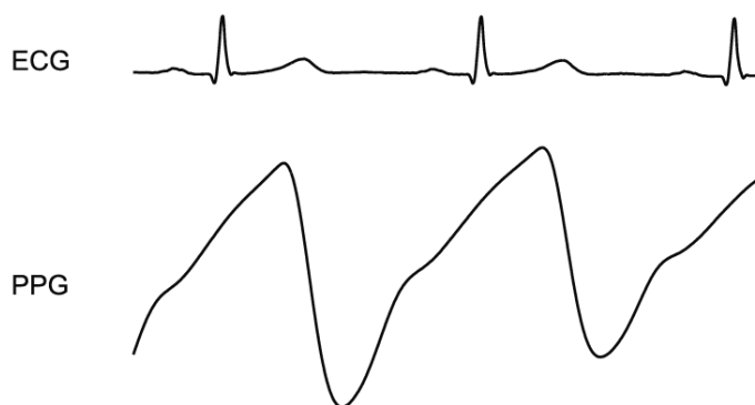
Figure 5- The pulsatile (AC) component of the PPG signal and corresponding electrocardiogram (ECG) [15].
