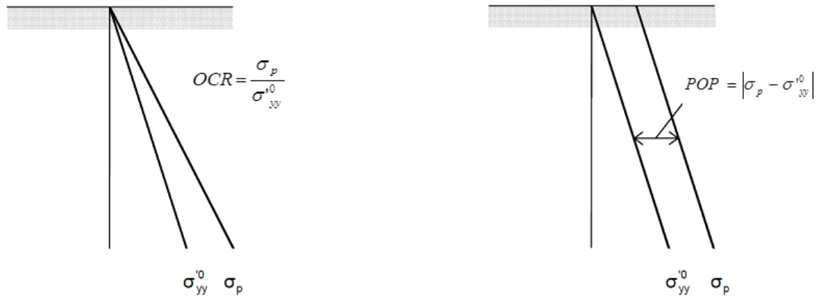
Figure 6.7 – Illustration of vertical preconsolidation stress in relation to the in-situ vertical stress using OCR and POP (Plaxis, 2006)
