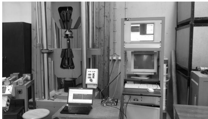
Figure 3.21 - Bolts strain gauges calibration set-up
