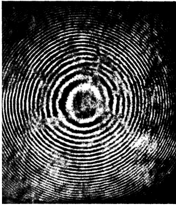
Figure 1.7: Interference phenomenon observed when the Fabry-Perot plate distance matches the optical length of the eye. [5]
