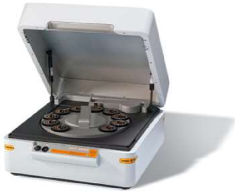
Figure 6. X-ray fluorescence spectrometer scattered energy (EDXRF), Epsilon 3 XLE , bench used in this study (adapted from http://www.panalytical.pt/Epsilon-3XLE.htm ).
