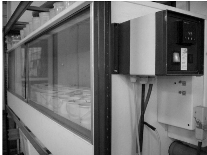
Figure 7. Extraction of soil microarthropods using Berlese Tullgren method
