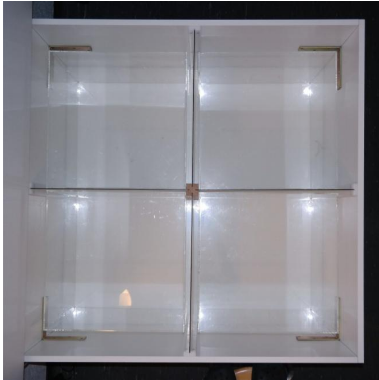
Figure 2.3 – Top view of the open field apparatus. Four plexiglas adjacent boxes are separated with wood dividers to avoid animals' eye contact, and placed over an infrared light. A ceiling hanging infrared camera captures the movements of the multiple subjects and sends the data to a PC for storage and analysis.
