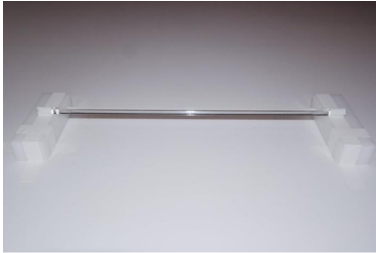
Figure 2.5 – Bar test apparatus. The 4 cm elevated acrylic bar and both plastic bases were fixed to the surface with white tape. The test is done facing a wide black curtain.
