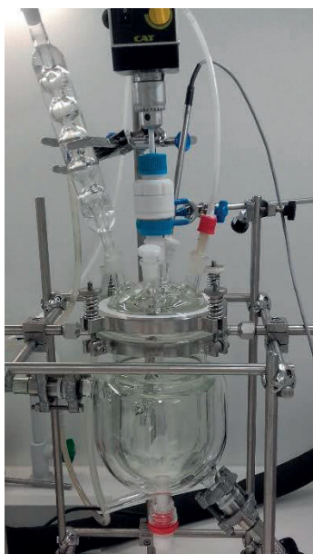
Figure 4.1: Experimental setup for the production of microcapsules by suspension polymerization available at Devan-Micropolis.
