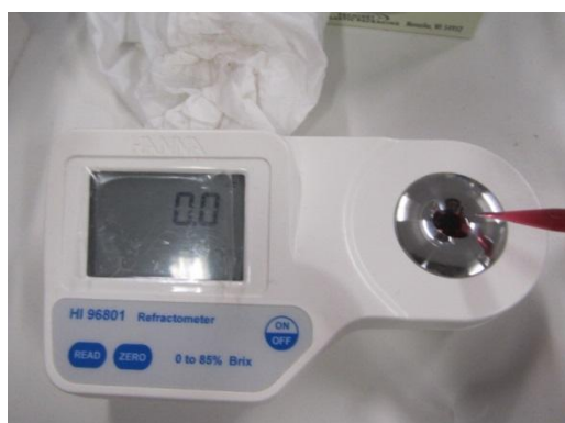
Figure 15 | Refractometer used in the measurement of °Brix of the different blueberry treatments.
