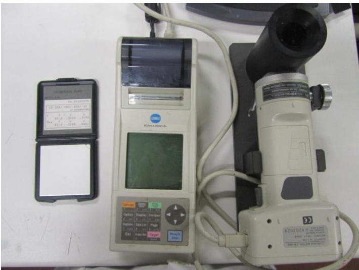
Figure 17 | Colorimeter used for color characterization of blueberry pulp, to the different treatments over time.
