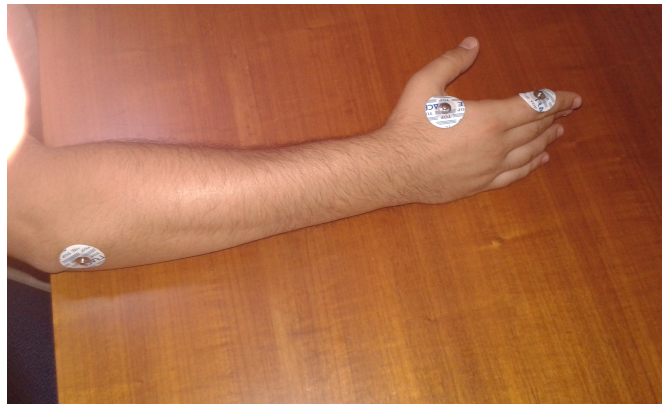
FIGURE 2.1: EMG Setup for FDI MEP measurement
