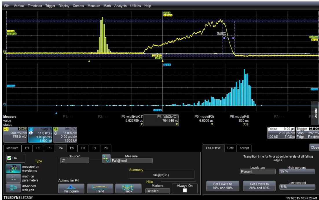
Figure 4.26. Signal output and histograms of the fall time (cyan) and full time (yellow) obtained with a driftless GPSC, for the mixture of 99.89% Xe+0.11% CO 2 , for a reduced electric field, E/p, of 2.55V/cm/torr.
