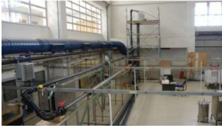
Figure V.2 – Pilot rig existent in DEQ-FCTUC without the EIT system (adapted from Rasteiro (2011)).
