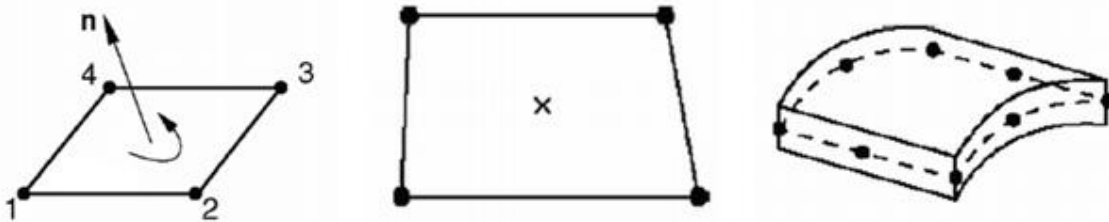
Figure 5.1 Schematic representation of the S4R element (Abaqus Analysis – User’s manual, 2012.)
