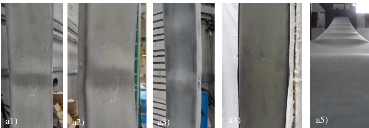
Figure G.13 Different configurations due to sectional buckling modes (local and distortional buckling) observed in the experimental tests.
