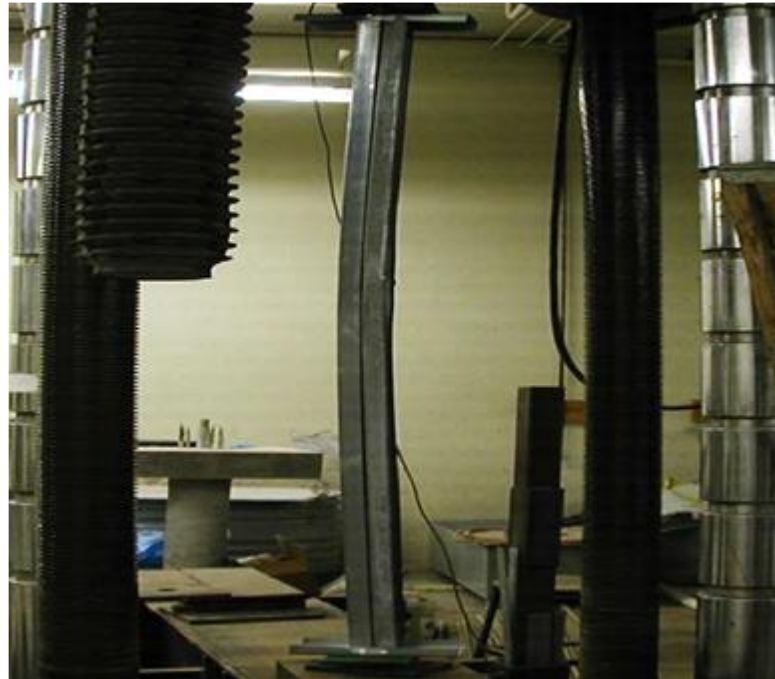
Figure 2.29 Failure observed for the open built-up I cross-section (Stone and LaBoube, 2005).
