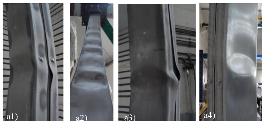
Figure G.21 Different configurations due to sectional buckling modes (local and distortional buckling) observed in the experimental tests.
