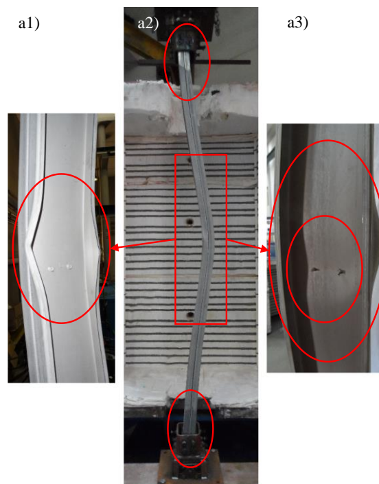
Figure 4.58 Failure modes for the specimen I_SR_50LL_K3-2. a1) and a3) Distortional buckling. a2) Flexural buckling.
