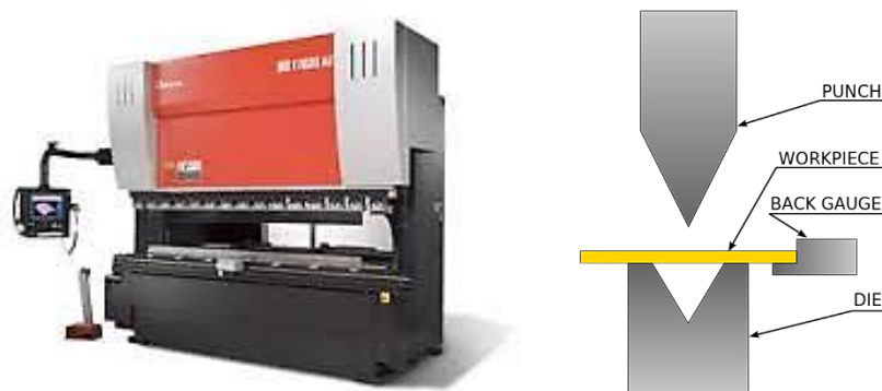
Figure 1.4. Press braking machine (Amada America, Inc@, 2015).
