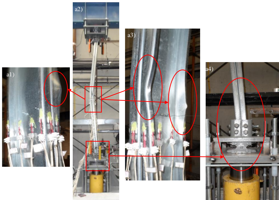
Figure 4.50 Failure modes of the test column I_FF_2 at ambient temperature. a1) and a3) Distortional buckling. a2) Flexural buckling. a4) End-support device.
