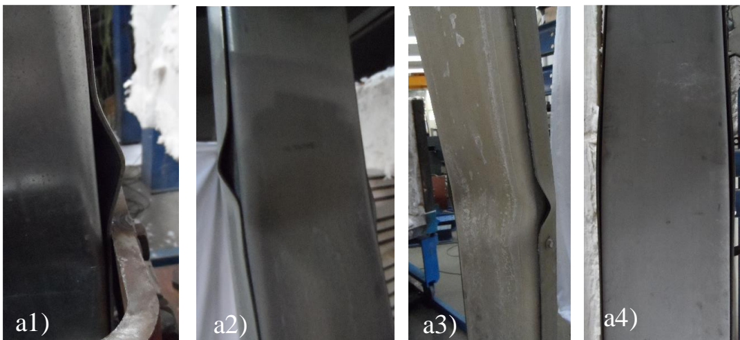
Figure G.19 Different configurations due to sectional buckling modes (local and distortional buckling) observed in the experimental tests.
