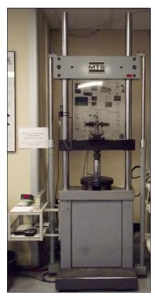
Figure NB.1. MTS tension-compression hydraulic machine.
