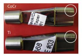
**Figure 1.6.** H-Max neck adapters after mechanical testing. In the laterodistal area of Ti neck adapters slight scratches could be observed (bottom). No surface damages at the Co-Cr neck adapters were seen (top) [13].
