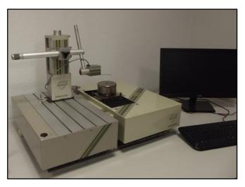
Figure 2.8. Two dimensional contact profilometer.
