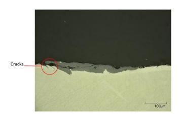
Figure 3.31. Image of a transversal wear scar taken by Keyence microscope with an amplification of 300x. Indication of the localization of the cracks. Test conditions: flat with normal roughness subjected to 1000 N of normal force, a displacement amplitude of ±30 µm and 50.000 cycles. This test is in partial slip regime given the, almost perfect, elliptical shape of the log (Figure 3.30).
