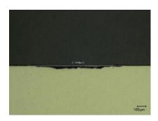
Figure 3.23. Image of a transversal wear scar taken by Keyence microscope with an amplification of 300x Test conditions: flat with normal roughness subjected to 600 N of normal force, a displacement amplitude of  $\pm 40 \ \mu m$  and 50.000 cycles.
