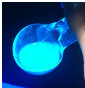
Figure 2.14: Image of the reaction mixture after the “click” reaction between the alkyne functionalized PDPA and N 3 -Cum. The formation of the fluorescent linkage could be easily seen upon irradiation at 365 nm with a hand-held UV lamp.
