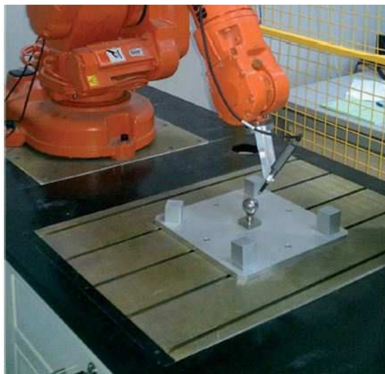
Figure 2.12 Calibration structure with a ball and a cube [41]
