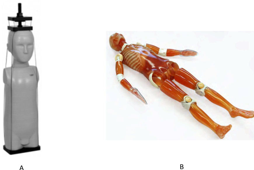
Figure 23: Anthropomorphic phantoms used in experimental tests A - Phantom CIRS™ ATOM model 705; B- Phantom Kyoto kagaku™ model PBU-60
