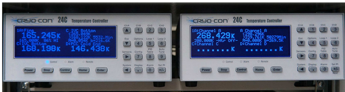
Figure 3.9 – A pair of Cryo-con, Inc. Model 24C Cryogenic Temperature Controllers. Left one is used for WILiX while the right is one used for the GPM temperature control.
