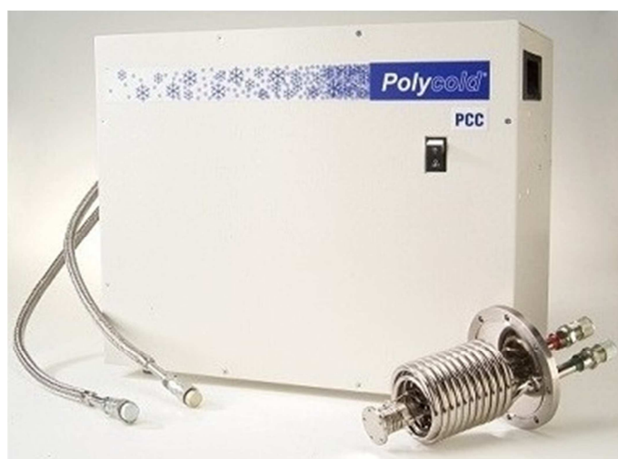
Figure 3.6 – Brooks Automation Polycold PCC Cryotiger compressor, supply and return lines of the refrigerant gas and cryocooler.
