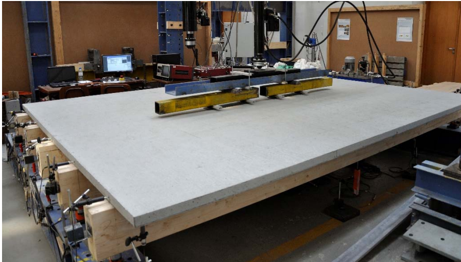
Fig. 4.16 – Test setup: four-point load at S1-BSp
