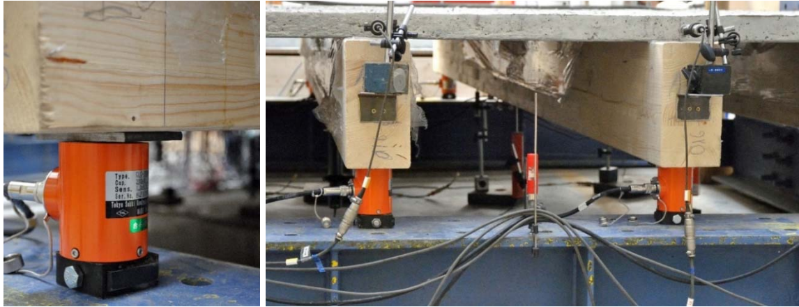
Fig. 4.25 – Test setup detail: load cells
