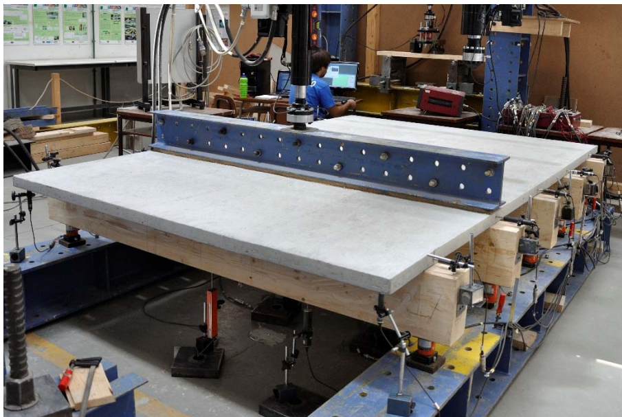
Fig. 4.19 – Test setup: line load at the 2.00 m span specimen (S4-L=2.00m)
