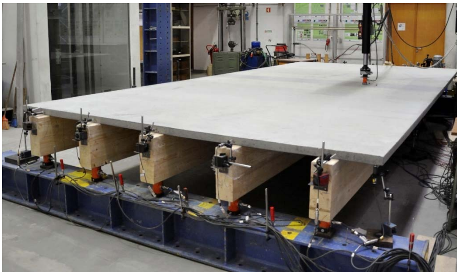
Fig. 4.14 – Test setup: ½ point load (S5-L=6.00m)
