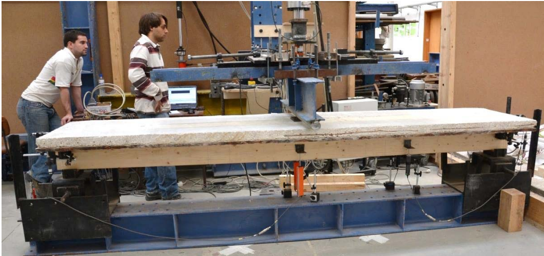
Fig. 3.13 – Beam (GL7) obtained from the CSGL slab subjected to a load test
