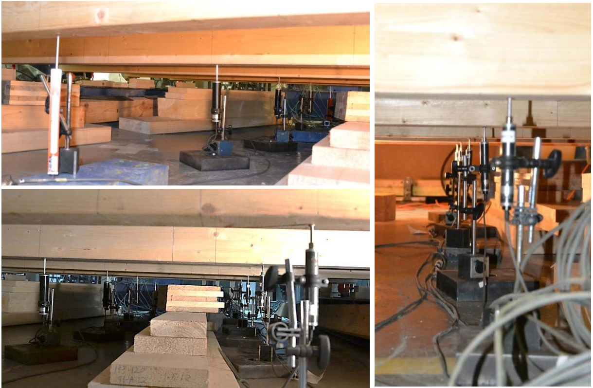
Fig. 3.6 – Test setup detail – CSGL: vertical displacement transducers
