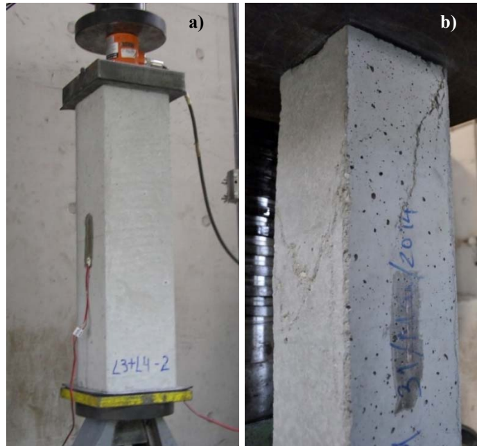
Fig. 4.3 – Testing of prismatic concrete specimens: a) MOE; and b) failure
