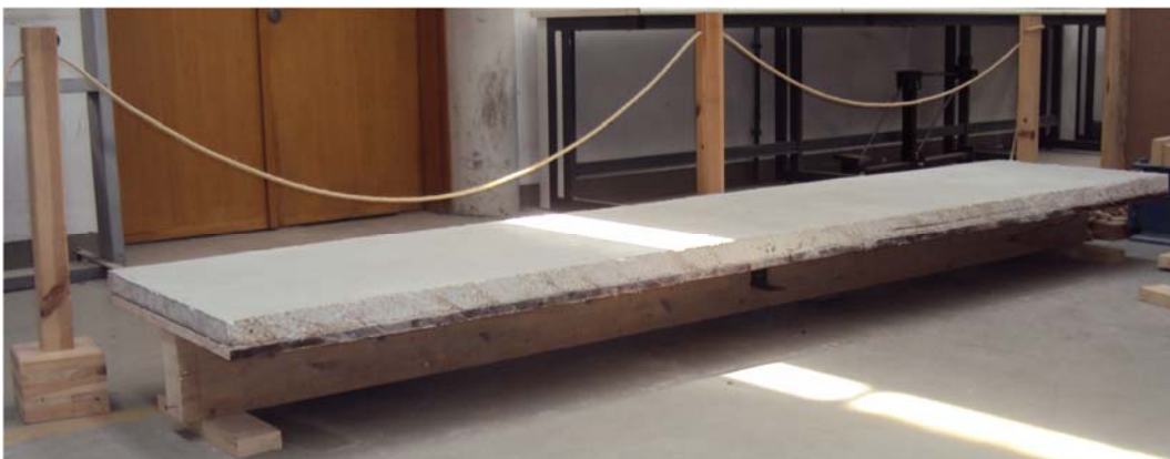
Fig. 3.12 – Composite T-beam obtained from the CSGL slab
