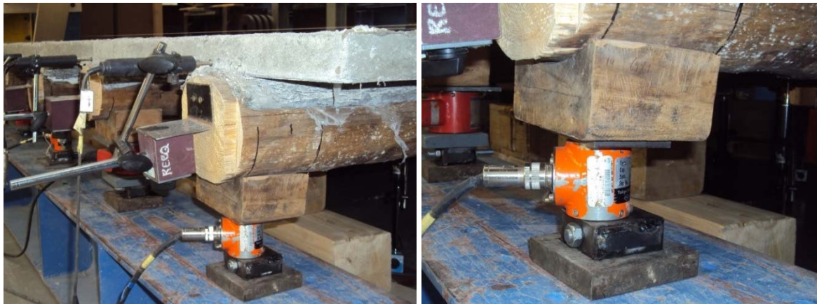
Fig. 3.10 – Test setup detail – CSTL: load cells
