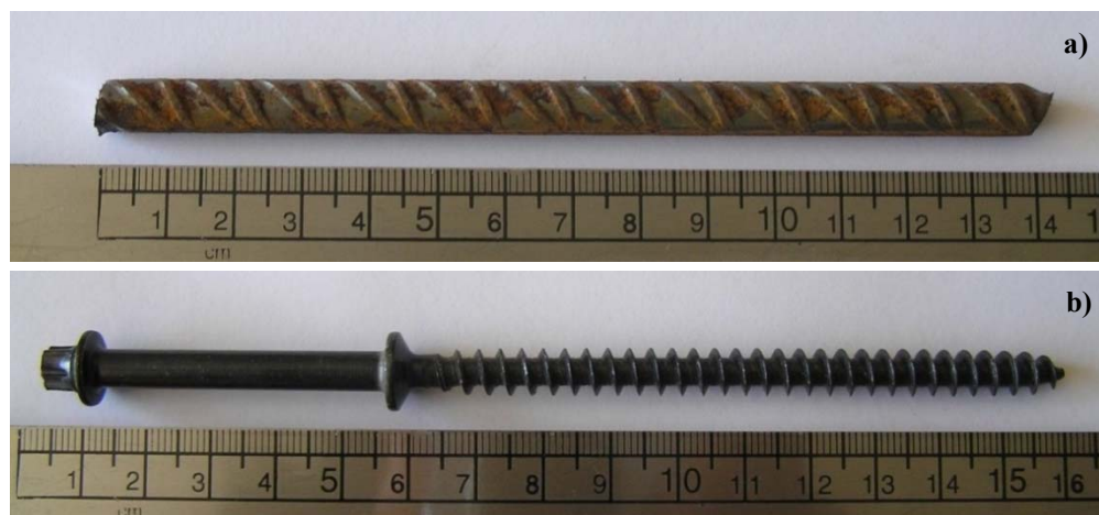
Fig. 4.5 – Connectors: a) steel rod \varnothing 8 mm; and b) SFS VB 48-7.5x100 screw
