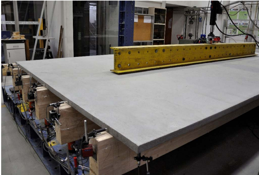
Fig. 4.20 – Test setup: line load at the 6.00 m span specimen (S5-L=6.00m)
