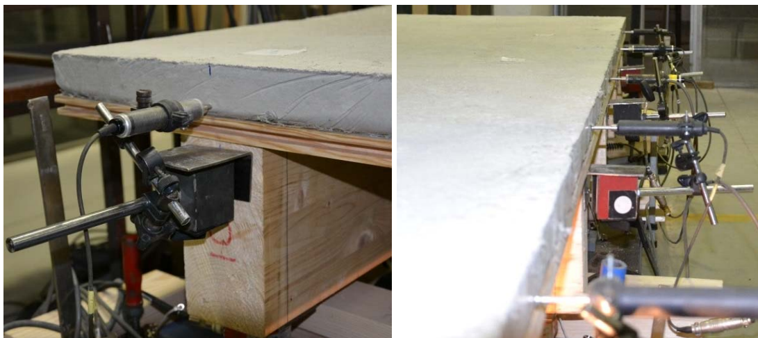
Fig. 3.5 – Test setup detail – CSGL: slip displacement transducers
