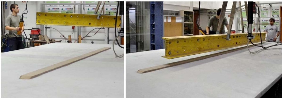
Fig. 4.17 – Test setup: line load regularization layer detail (S5-L=6.00m)
