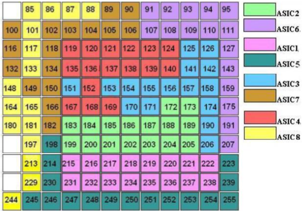
Figure 5.5: Pixel association with the 8 ASIC channels. Pixel numbers start at 85 because not all the matrix is being used.
