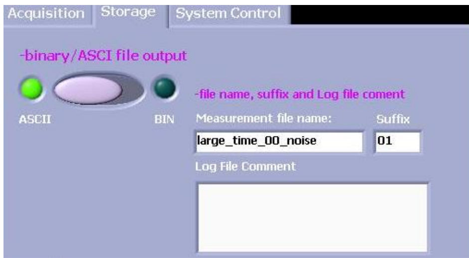
Figure 5.9: Storage interface of the LabView S/W. It includes a switch in top left side that dictates the data type of the stored information and three text boxes where the name of the file, suffix and comments can be inserted.
