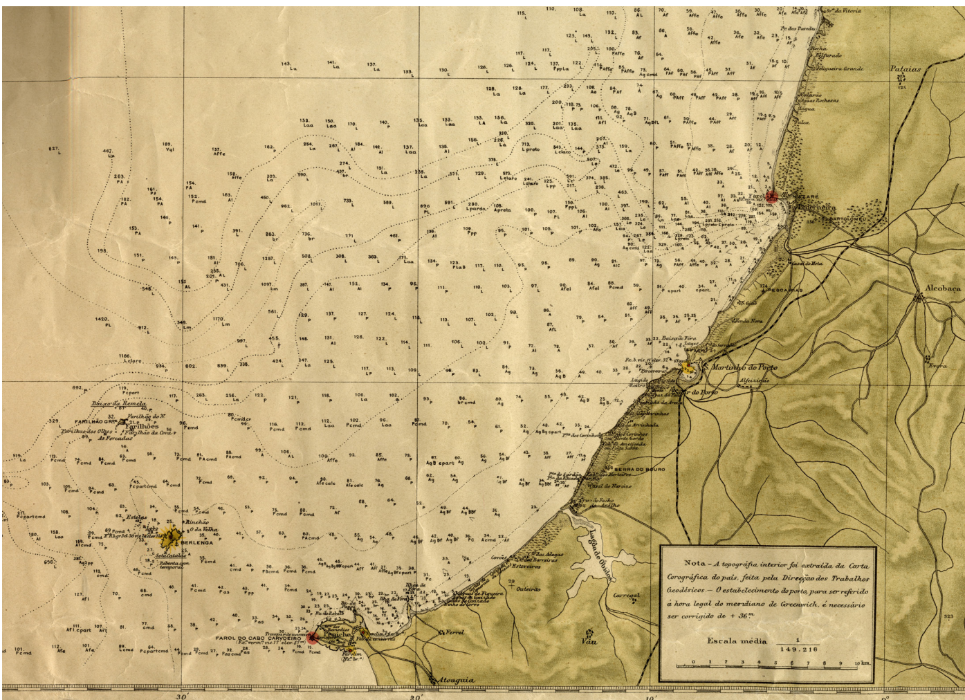
Fig. 3.9 - Map of central Portuguese coast with bathymetry offshore and topography onshore, 1:150 000 scale (date: 1915).
