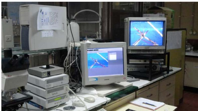
**Figura A1.4** PLTM (*Polarized Light ThermoMicroscopy*), *Hot Stage* DSC600 da Linkam.
