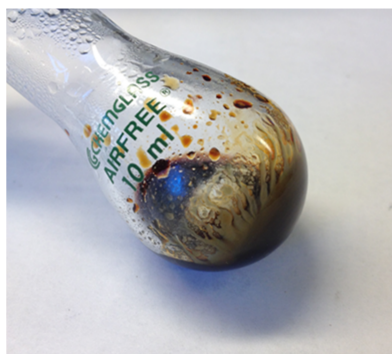
Figure B.4. Reaction mixture of the normal ATRP of AMA, at 91% monomer conversion, showing the precipitation of the polymer. Conditions: [AMA]_0/[EBiB]_0/[CuCl]_0/[bpy]_0 = 30/1/1/2 ; T = 50\text{ }^\circ\text{C} ; [AMA]_0 = 2\text{ M} ; V_{\text{total}} = 2\text{ mL}
