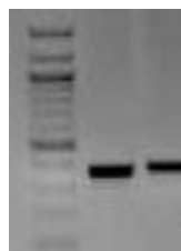
Figure 12 - Agarose gel showing the amplification of 3'UTRs of FoxO1 in the first lane and FoxO3 in the second lane.
