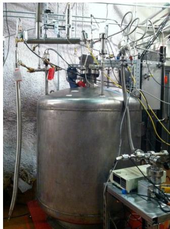
Figura 2.9: Safety Recovery Vessel (SRV).
