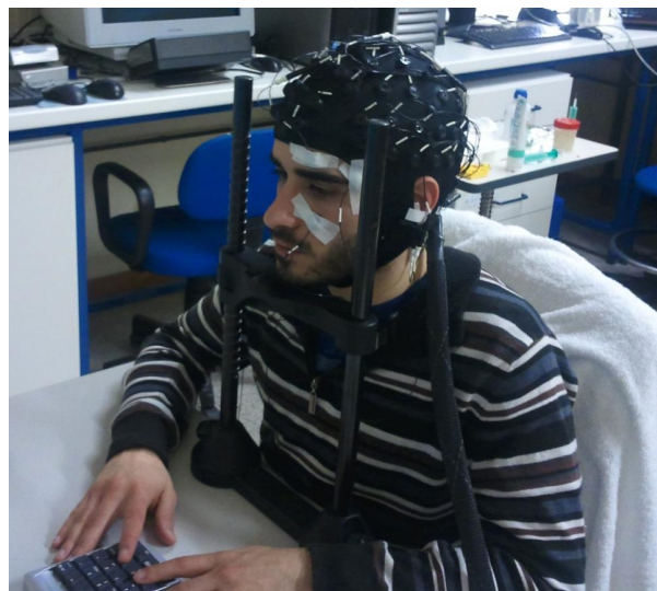
Figure 2.12: Example of a participant prepared for EEG acquisition correctly positioned for the eye-tracker monitoring his eyes.
