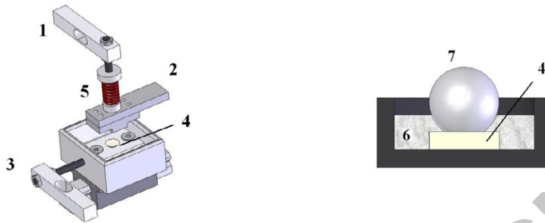
a) b) Fig. 1. Reciprocating equipment for sphere-plane contact; a) upper and lower specimen carrier, b) schematic of contact geometry and environment solution.
