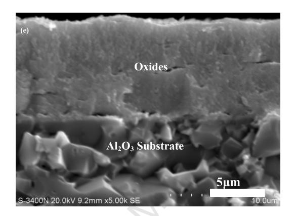
Fig. 7. TGA curves (a), SEM surface (b, d) and fracture cross-sectional micrographs (c, e) of the CrAlZr5N (b, c) and CrAlZr27N (d, e) coatings on  $Al_2O_3$  slices after thermal exposure at 900  $^{\circ}C$  in industrial air for 2h. Oxides are Cr-rich in (c) and Zr-rich in (e), respectively; Nitrides are (Cr, Zr)N phases in (c).
