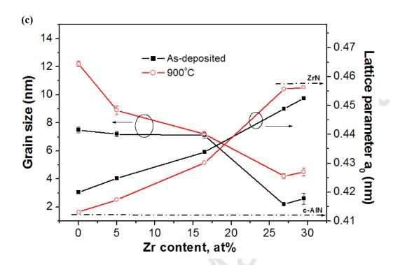
Fig 3. XRD patterns (a, b) and calculated grain size and lattice parameter (c) of the coatings on M2 steels as-deposited (a) and annealed at 900  $^{\circ}$ C in 95% Ar + 5% H<sub>2</sub> atmosphere for 1h (b). The XRD tests were done with Co K $\alpha$  radiation ( $\lambda$  = 0.178897 nm) in grazing mode (2 $^{\circ}$ ). CrN (ICDD 11-0065), ZrN (ICDD 35-0753), Cr (ICDD 85-1336), *t*-ZrO<sub>2</sub> (ICDD 50-1089).
