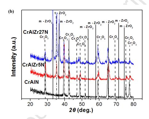
Fig. 6. TGA curves (a) and XRD patterns (b) of the coatings on  $Al_2O_3$  slices thermally exposed to 1200 °C in industrial air (99.995% purity) for 1h. The XRD tests were done with Co K $\alpha$  radiation ( $\lambda$  = 0.178897 nm) in grazing mode (2°).  $Cr_2O_3$  (ICDD 38-1479), m-ZrO<sub>2</sub> (ICDD 17-0923), t-ZrO<sub>2</sub> (ICDD 50-1089).
