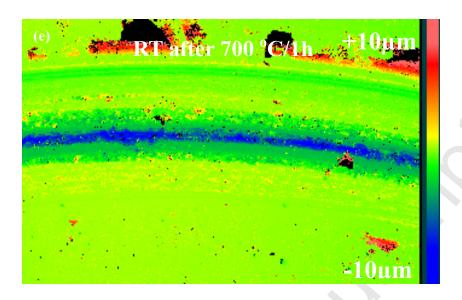
Fig. 9. Friction coefficient (a), wear track profile (b) and surface morphologies (c, d, e) of the CrAlZr27N coating on M2 steel testing under different conditions. 5 N normal applied load, 5 cm/s sliding speed and 5000 laps, and 6 mm Al<sub>2</sub>O<sub>3</sub> ball as a counterpart.
