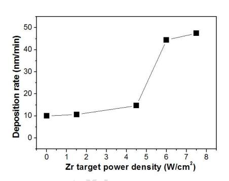
Fig. 1. Deposition rate of the coatings deposited with increasing Zr target power density.
