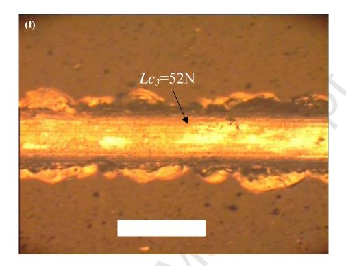
Fig. 5. Typical scratch track morphologies of the coatings on M2 steels as-deposited (a, c, d) and after 900  $^{\circ}$ C annealing (b, e, f): (a, b) CrAlZr5N; (c, d, e, f) CrAlZr27N. 200  $\mu$ m tip radius indenter, 100 N/min loading speed and 10 mm/min scratch speed. Scratch direction is from left to right. The arrows point out the positions of coating failure during scratching.  $Lc_2$ - edge chipping,  $Lc_3$ - substrate exposure.
